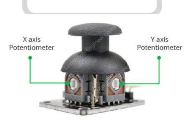
The two gray boxes on either side of the joystick are the potentiometers. If you move the joystick while keeping an eye on the potentiometer, you'll notice that each potentiometer only detects movement in one direction.
