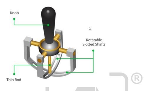
Each shaft is connected to a potentiometer so that moving the shaft rotates the corresponding potentiometer's wiper. In other words, pushing the knob all the way forward will cause the potentiometer wiper to move to one end of the resistive track, and pulling it back will cause it to move to the opposite end.
