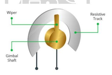
The joystick outputs an analog signal whose voltage varies between 0 and 5V. When you move the joystick along the X axis from one extreme to the other, the X output changes from 0 to 5V, and the same thing happens when you move it along the Y axis. And, when the joystick is centered (rest position), the output voltage is approximately half of VCC, or 2.5V.
